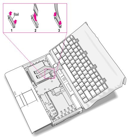
1 Slide the keyboard forward and position it with the tabs at the top sliding into the enclosure.
